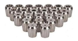
DESIGN: ER collets are cylindrical in shape and consist of a threaded outer surface that allows them to be screwed into a corresponding collet chuck or tool holder. They have multiple slits or slots along their length, which enable them to compress when tightened, effectively clamping onto the tool shank.
